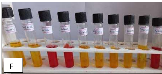
Photograph 3: Results of sugar fermentation test of yeast isolates. E- sugar fermentation test of Saccharomyces cerevisiae Ch1 F- sugar fermentation test of Saccharomyces spp Pn4.
