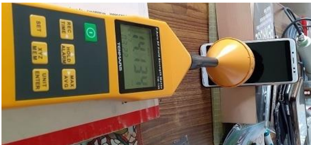
Fig. 1: Experimental set up: Recording of the electric field of a cell-phone by TM-196
