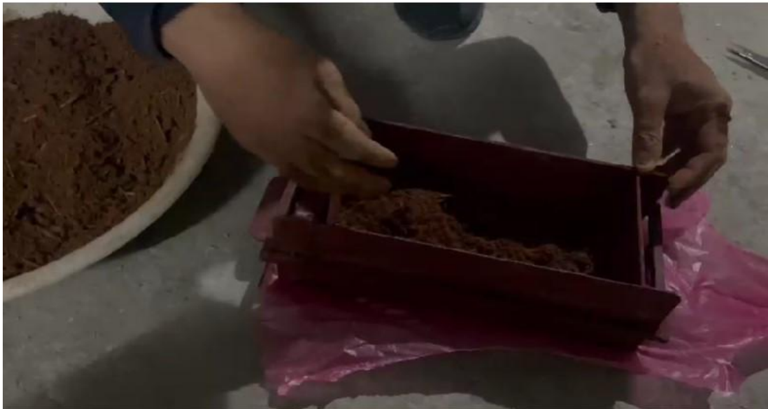
Figure 4: Placement of mixture in mould
