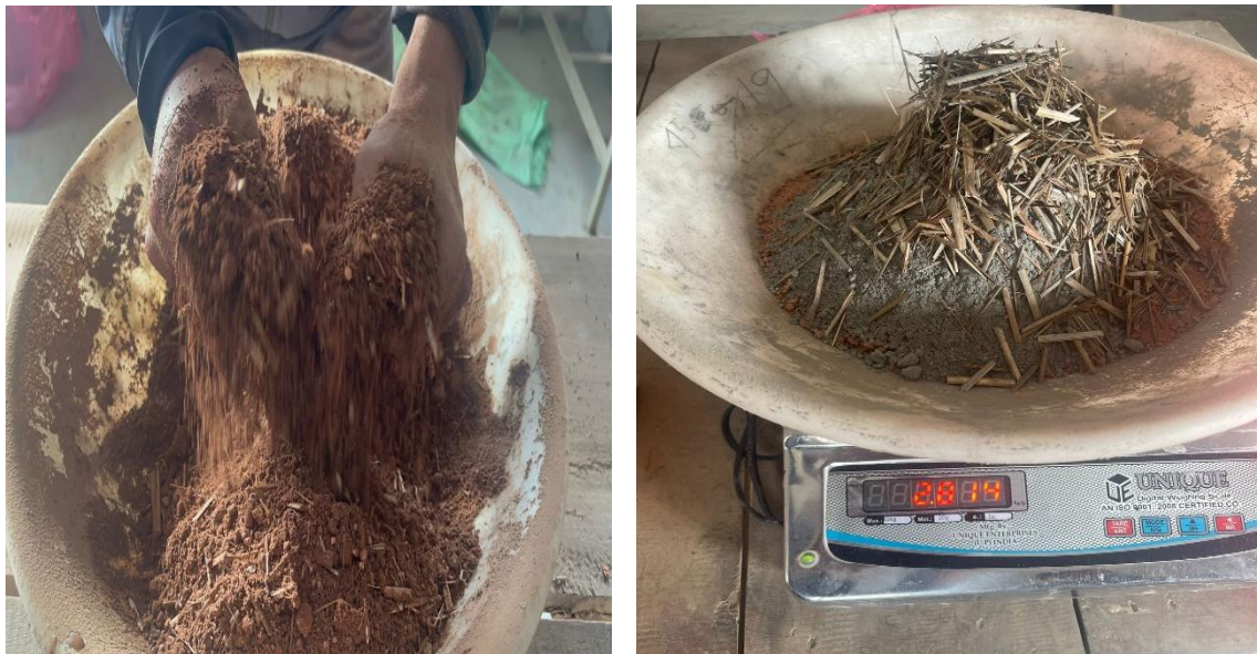
Figure 1: Sample weighting and Hand mixing
