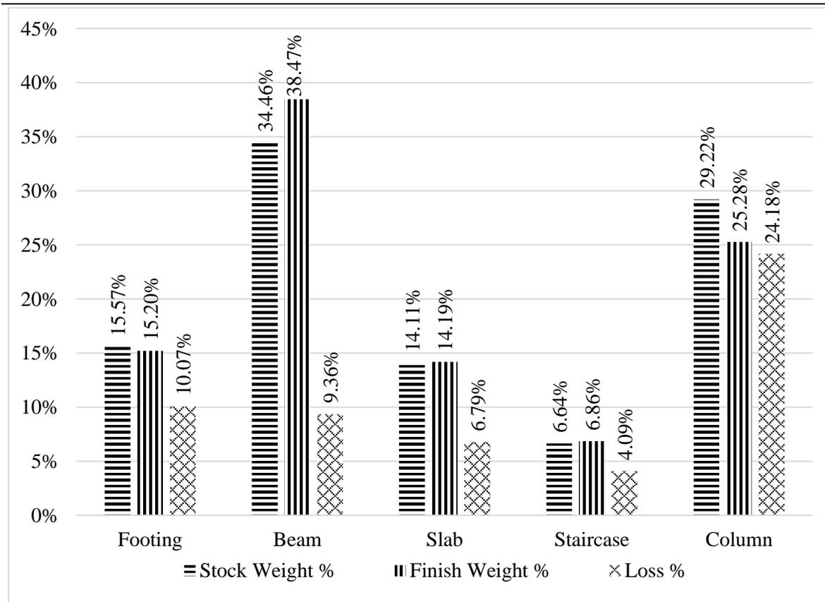
**Figure 5:** Cutting waste by structural components in 3-C-7.
