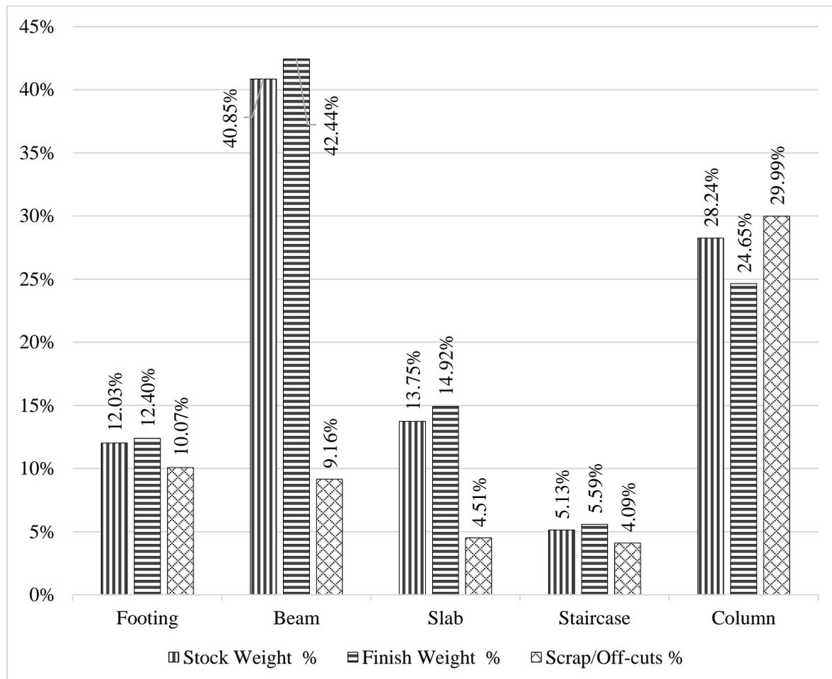
**Figure 4:** Cutting waste by structural components in 3-C-9
