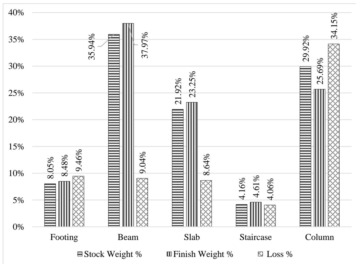
Figure 6: Cutting waste by structural component in 4-C-16
