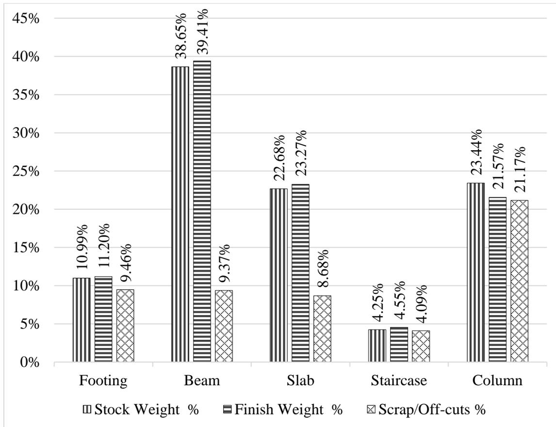
Figure 3: Cutting waste by structural component in 3-C-12.
