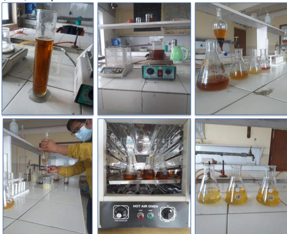
Fig. 40. Transesterification process of biodiesel preparation
