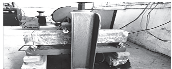
Fig. 5: Flexure strength test of beam
