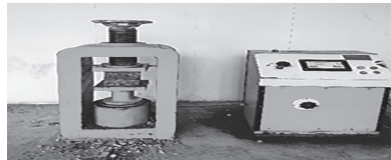
Fig. 3: Compressive strength test of block
