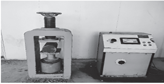
Fig. 4: Split tensile strength test of sample
