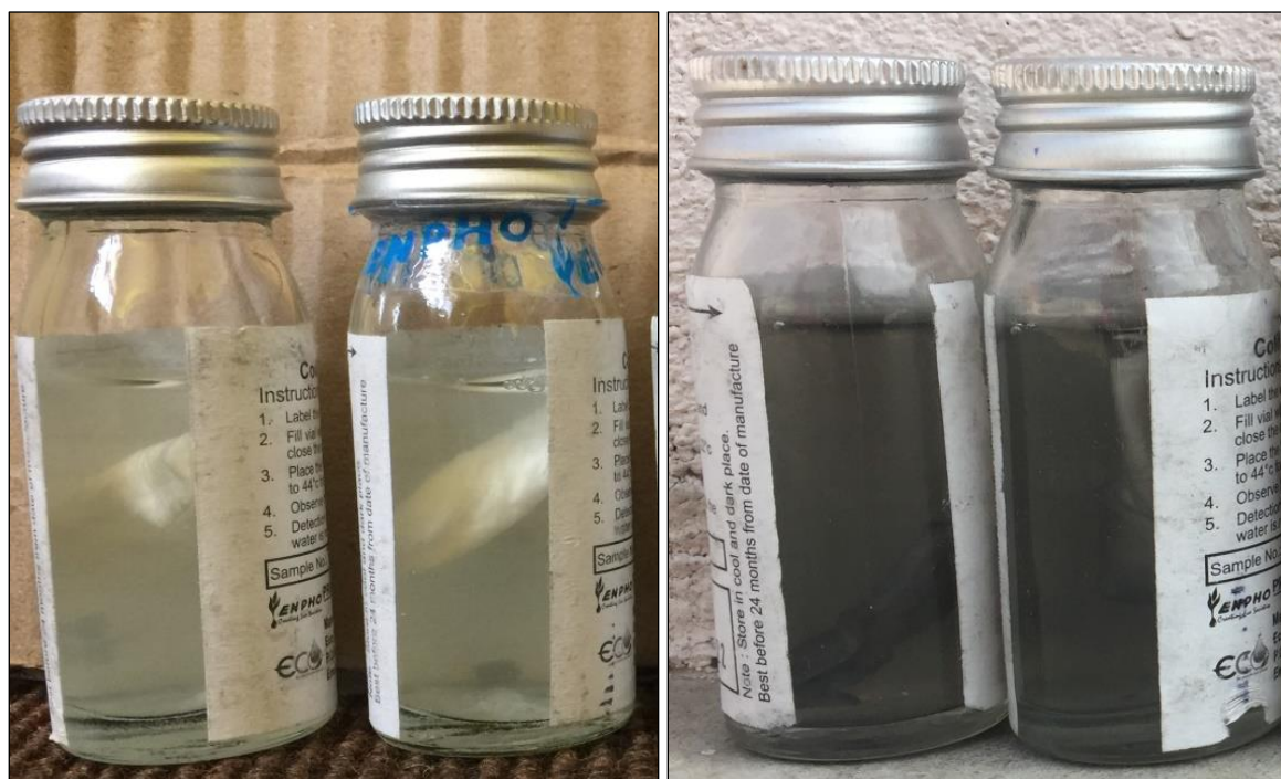
Figure 3: Coliform presence/absence (H 2 S) test vials after 48-hour incubation. Left: Negative result (no color change), Right: Positive result (black coloration indicating fecal contamination).
