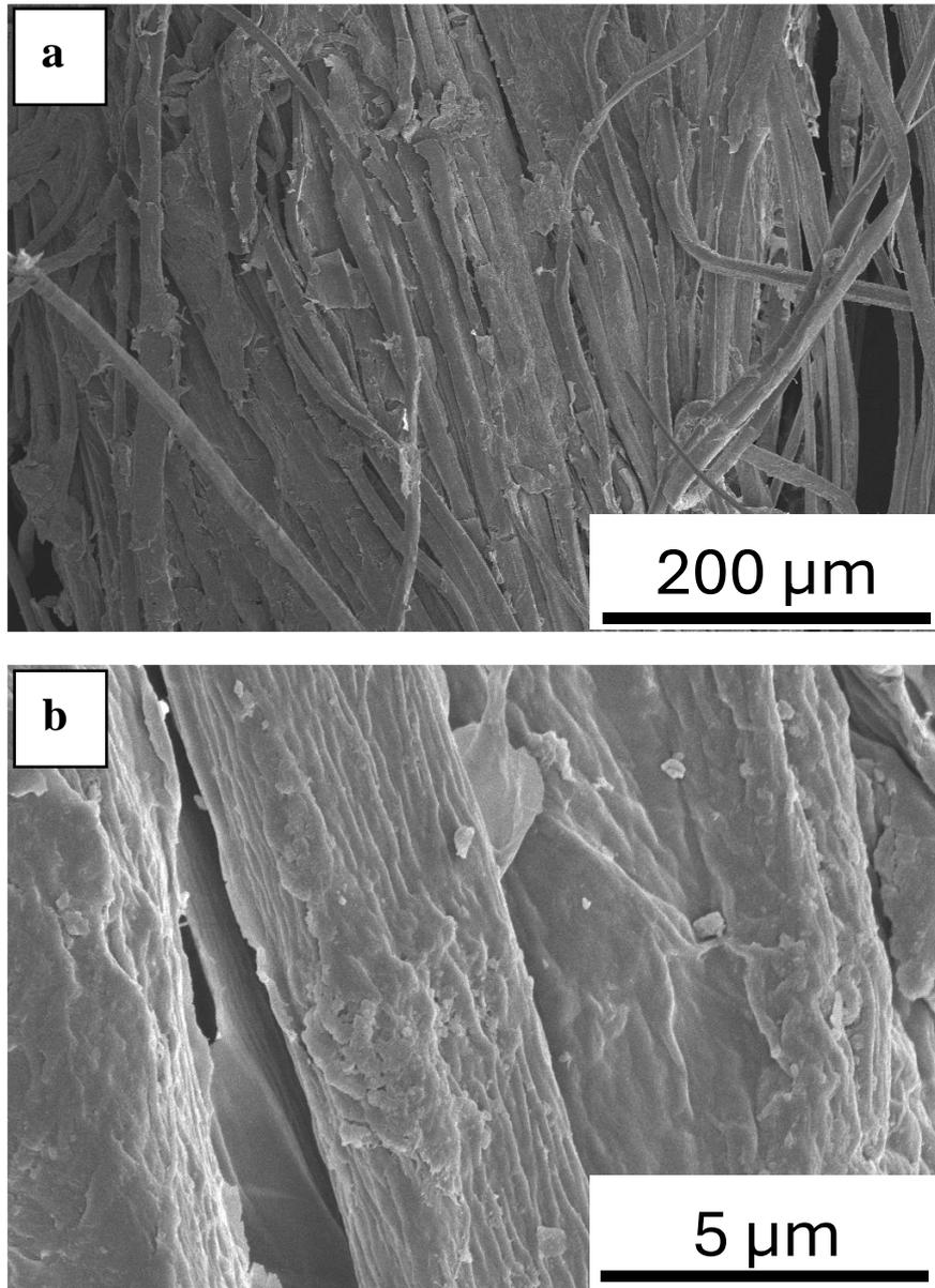
**Figure 3** Lower (top) and higher (bottom) magnifications of the scanning electron micrographs showing the detailed morphology of Argeli fiber
