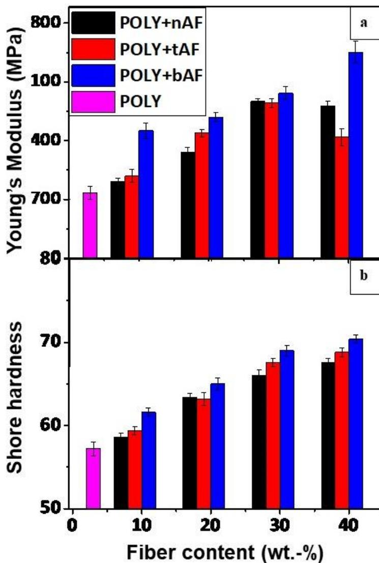
**Figure 5** Variation of tensile Young's modulus (a) and Shore D hardness (b) of the polymer blend as a function of Argeli fiber content as filler; POLY: polymer blend matrix; nAF: neat fibers prepared by mechanical processing; tAF: alkali-treated fibers; and bAF: bleached fibers
