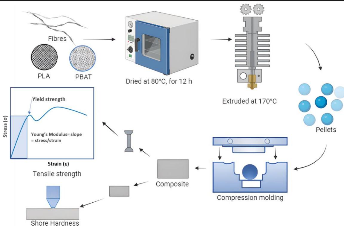
**Figure 2** Schematic illustration showing the experimental design for preparation of polymer composite and their analyses (prepared partly using the BioRender software)
