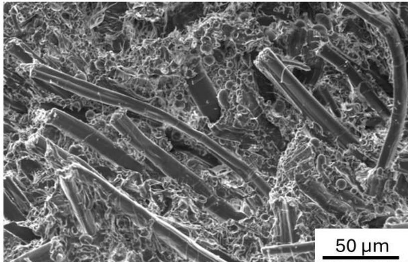
**Figure 4** Representative SEM image showing the fracture surface morphology of a composite comprising 20 wt.-% of Argeli fiber and 80 wt.-% biodegradable polymer blend (POLY)
