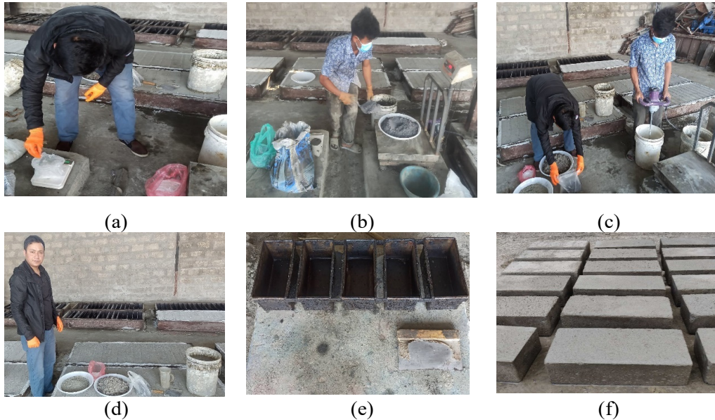
Figure 2 Raw Materials to CLC Block Production Unit (a)- weighing the ingredients, (b)-mixing the ingredients, (c)-mixing water to mortar, (d)-Checking the mortar, (e)-Preparing Molds, (f)-Manufacturing CLC blocks for curing
