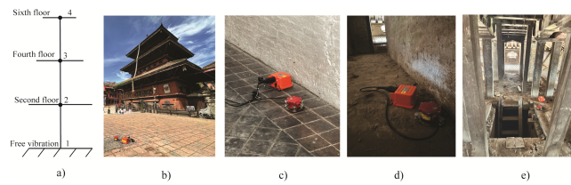
Figure 4. Multiple point measurement a) Illustrative diagram of the measured location, b) free-field, c) second floor, d) fourth floor, and e) sixth floor
