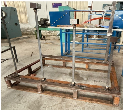
Figure 1: Experimental setup showing physical arrangement of the four SDOF System Prepared in Kathmandu University Structural Engineering Laboratory
