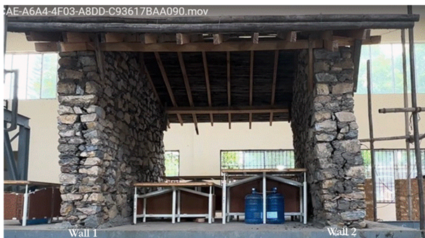
Figure 10. Initial pendulum impact (Shock #7) generates shear in walls and produces vertical crack separating the wall wythes
