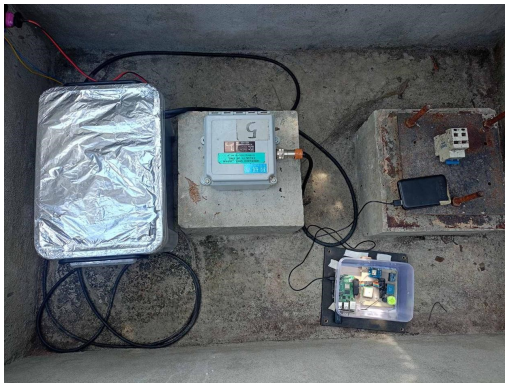
Figure 2. Seismometer setup for measurement and calibration
