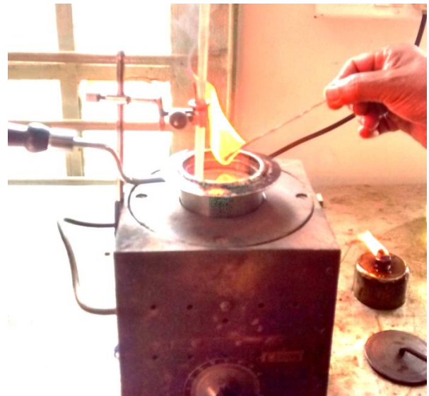
Fig. 4. Determination of fire point and flashpoint in laboratory
