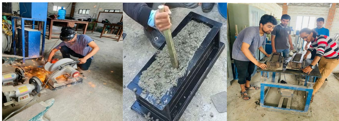
Figure 3: Cutting of steel Reinforcement for the Beam, preparation of the Beam and Compaction of the Beam Using a Vibrator
