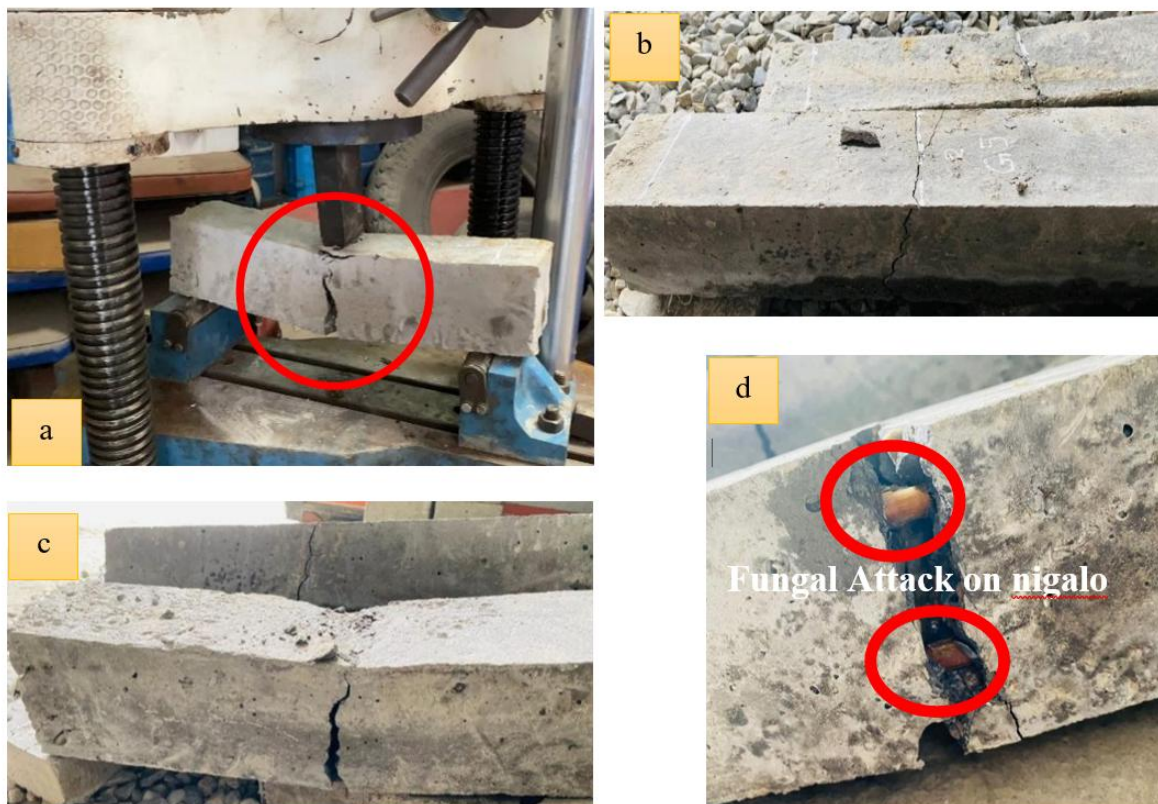
Figure 14: (a) Flexural testing of NRC Beam using UTM (b), (c) NRC Beam after testing (d) Degraded untreated Nigalo after 28 days of casting
