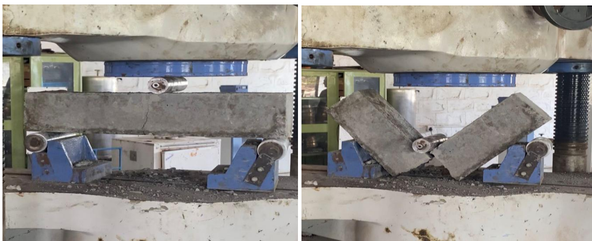
Figure 10: PCC beam showing crack formation during testing (left) and collapsed beam after failure (right)
