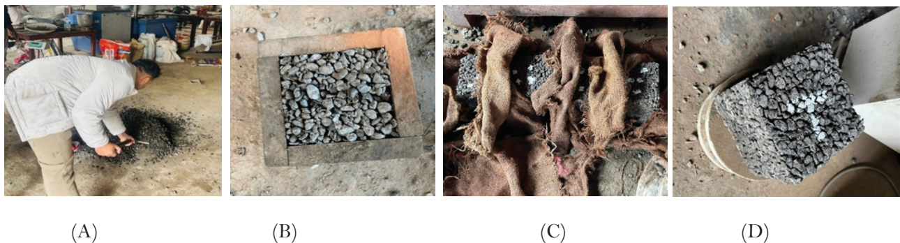
Figure 2: A) Hand Mixing B) Casting of cube in mould C) Curing with jute bag, D) Porous Concrete
