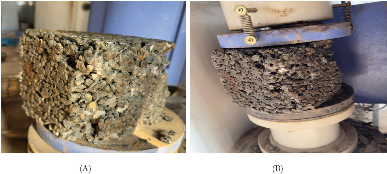
Figure 6: A & B development of cracks
