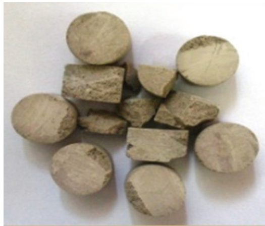
Figure 2: Porous bioactive glass Scaffold
