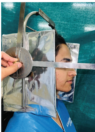
Figure 5: Horizontal arm of Goniometer axis passing through pupillary line and parallel to base of mandible.
