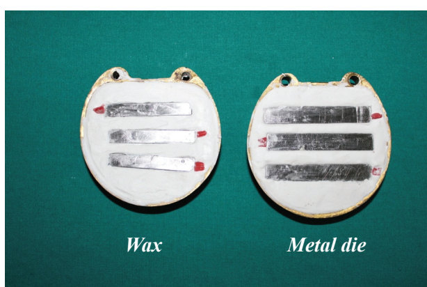
Figure 2: Flask with metal dies embedded in plaster for Group 1A, 1B, 2A, 2B
