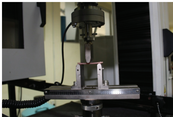
Figure 6: A prepared sample under flexural load
