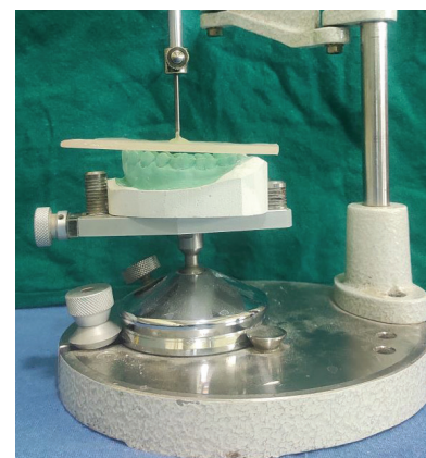
Figure 3: Cast Mounted in the Surveyor
