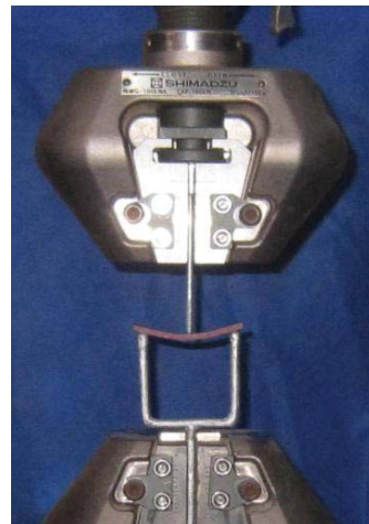
Fig 4: 3-point loading test in UTM
