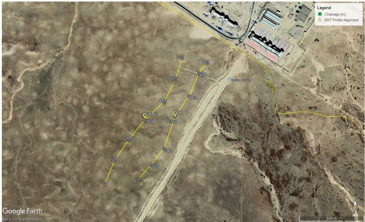
Fig. 3: Alignment of ERT Profile 1 and ERT Profile 2 (100 m apart, north-south orientation) relative to the Korala border crossing, shown on satellite imagery.
