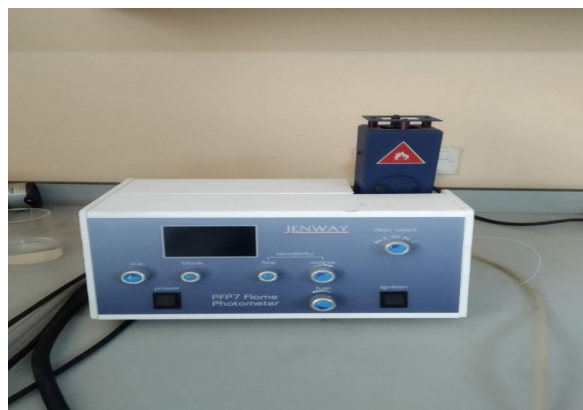
Fig. 2: Physiochemical parameters of the spring to determine WQI (a. Titration b. Flame Photometry)
