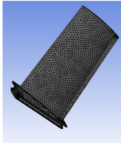
Figure 4: Finite element model of power turbine blade
