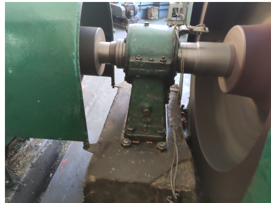
Figure 5: Bearing holding the shaft with the flywheel
