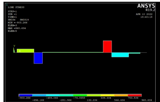
Figure 5: Shear force distribution along the shaft
