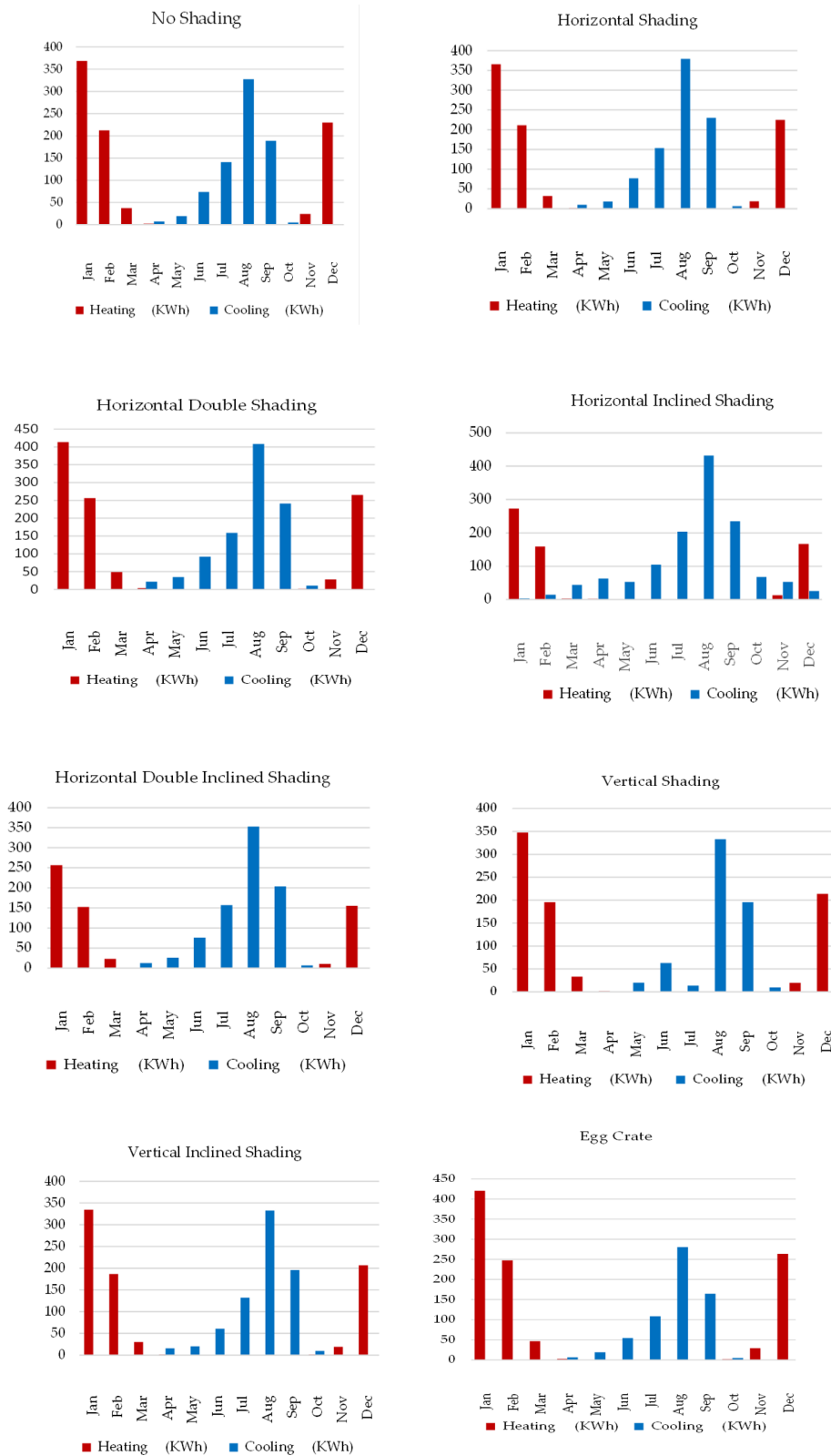
Figure 11: Showing heating and cooling loads in: No shading, Horizontal Shading, Horizontal Double Shading, Horizontal Inclined shading, Horizontal Double Inclined Shading, Vertical Shading, Vertical Inclined Shading, Egg Crate Shading. (The graph is the illustrative summary of the data result obtained from Ecotect)
