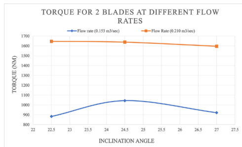
Figure 9: Torque vs. Inclination Angle in degrees for different flow rates for 2 bladed AST
