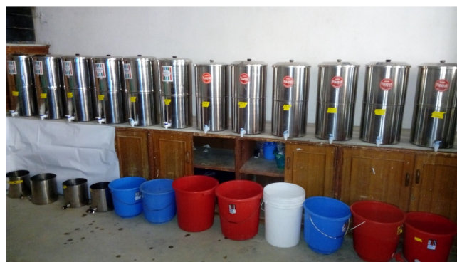
Figure 2: A photograph showcasing the filter setup for experimentation. Initially, 15 filters from five brands were utilized. In the second phase, two additional brands were incorporated, bringing the total to 21 filters from seven brands.
