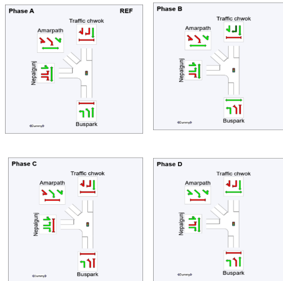
Figure 2. Phase sequence for Pushpal Chowk intersection for morning peak hour
