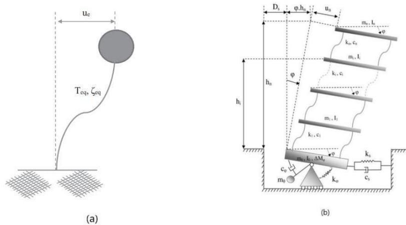
Figure 2 : (a) Equivalent SDOF fixed –base system (b) Non-linear soil-MDOF structure system [21]
