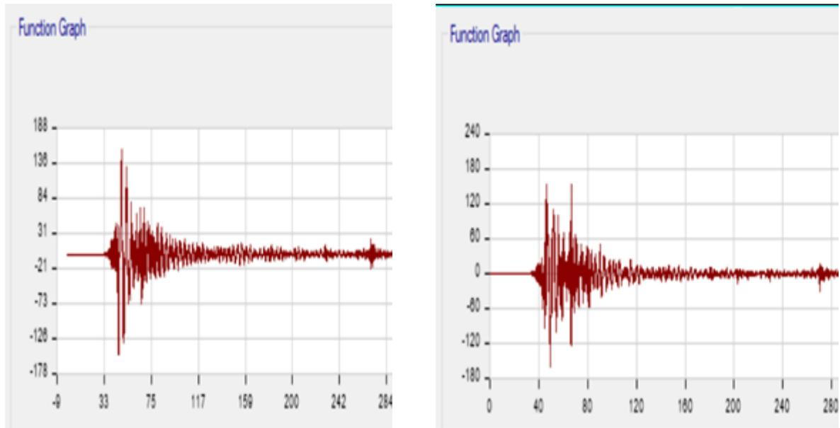
Figure 6: Time history graph of Gorkha Earthquake, along X-direction and along Y-direction
