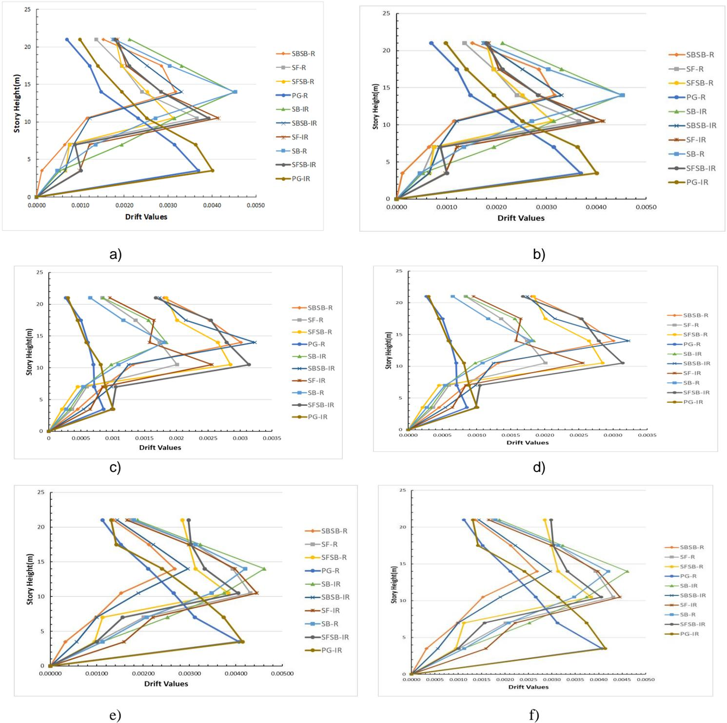
Figure 13: Distribution of Inter-Story Drift on Each Story for Fixed and Flexible Base Buildings Across Gorkha, Imperial, and Turkey Earthquakes (a-f)
