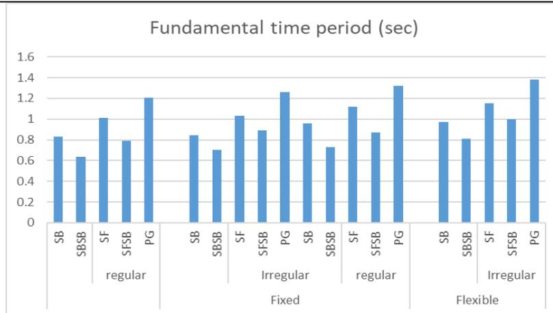
Figure 9: Comparison of fundamental time period for regular and irregular buildings
