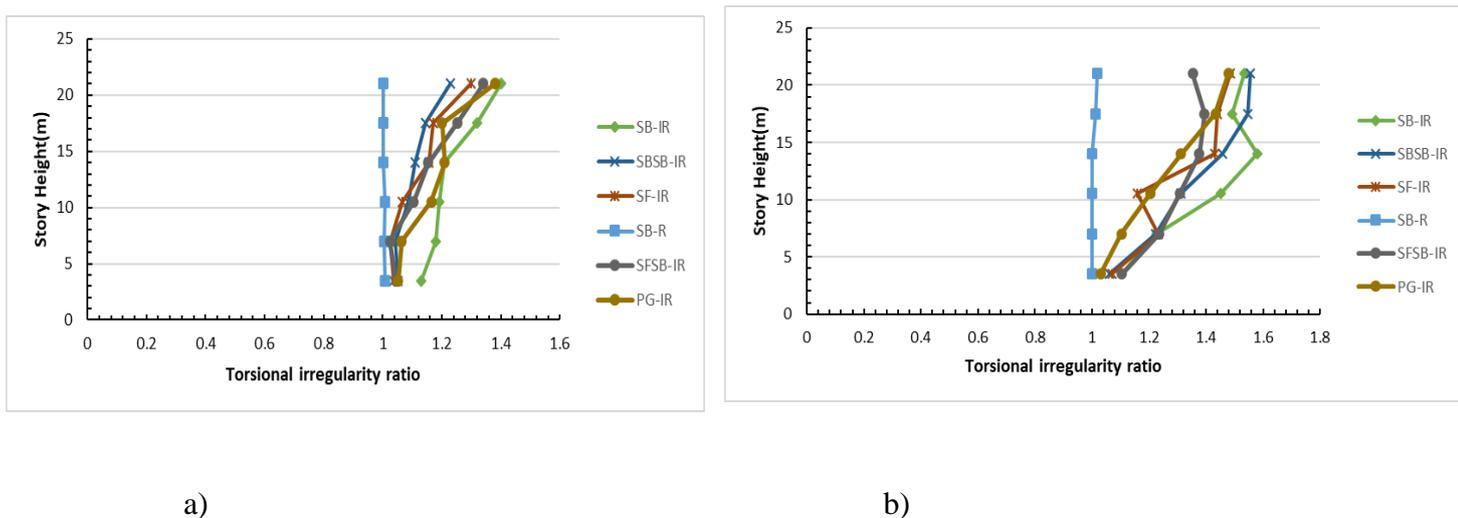
Figure 12: Torsional irregularity ratio along slope by response spectrum a) fixed and b) flexible base conditions
