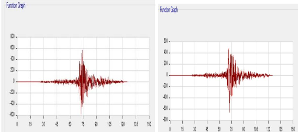
Figure 8: Time history graph of Turkey Earthquake, along X-direction and along Y-direction
