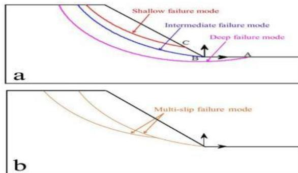
Figure 3: (a) Shallow, intermediate and deep failure (b) Multi slip failure [24]
