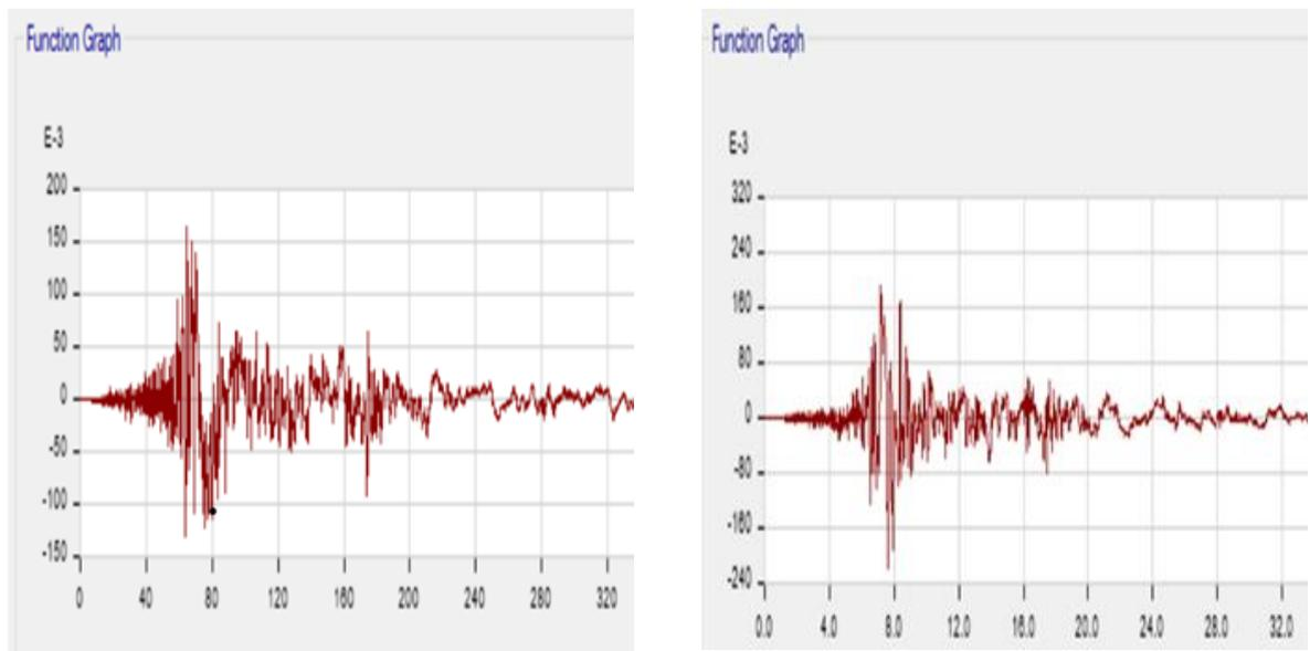
Figure 7: Time history graph of Imperial Earthquake, along X-direction and along Y-direction
