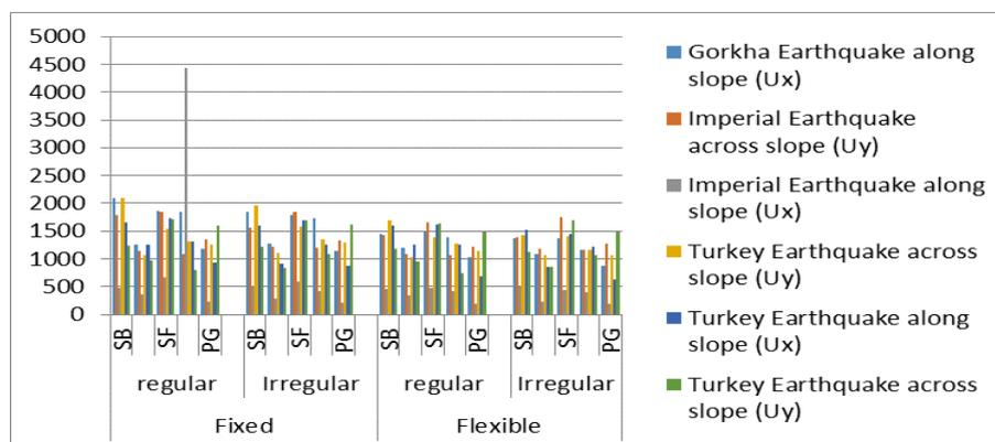
Figure 10: Base shear comparison for different building across slope for Gorkha Earthquake, Imperial Earthquake, and Turkey Earthquake
