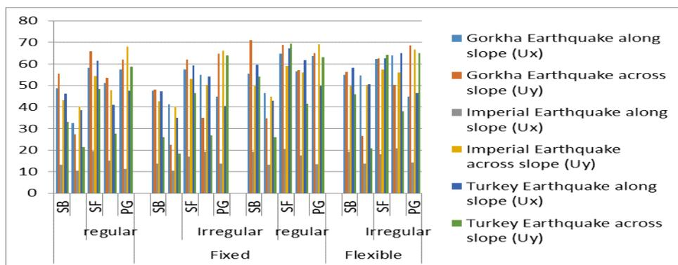
Figure 11: Comparison of top story displacement of different building with fixed and flexible base for Gorkha Earthquake, Imperial Earthquake and Turkey Earthquake
