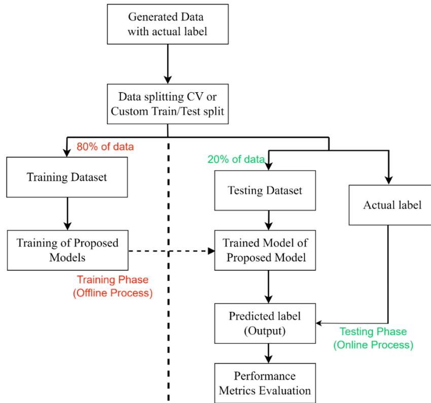
Figure 7: Flow chart of data training and testing based on proposed methods
