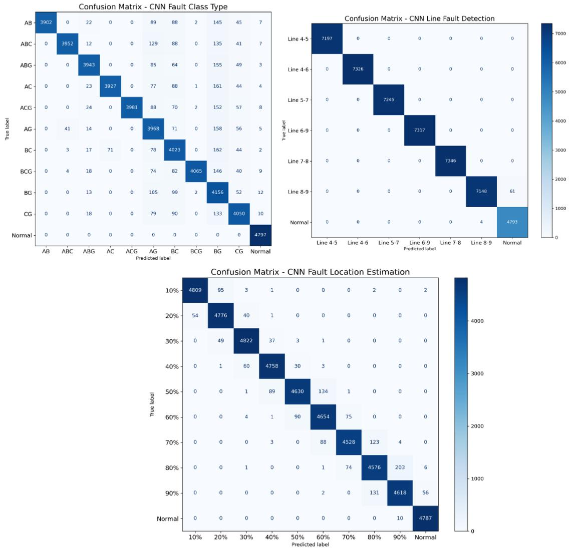
Figure 12: Confusion matrix of the Proposed CNN model
