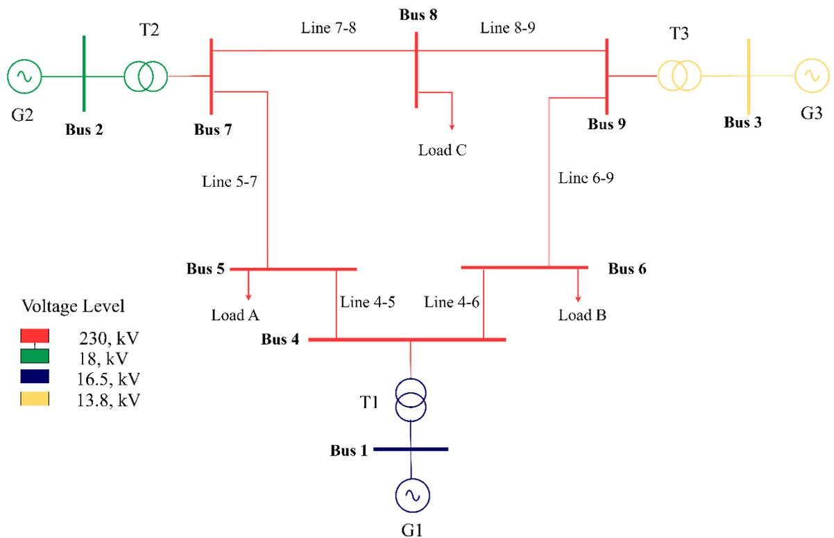
Figure 4: Single-line diagram of IEEE 9-Bus System
