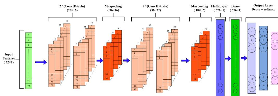
Figure 6: Architecture of the proposed 1D-CNN model
