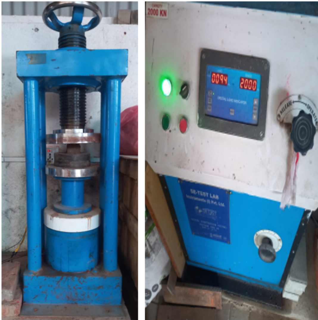
FIGURE 5. Test for compressive strength
