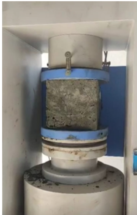
FIGURE 5. Preparation of Compression Test Specimens.
