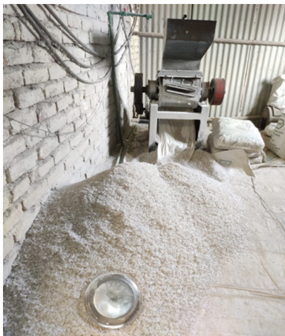
FIGURE 2. Shredding Machine for Powdered PET.
