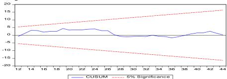
The green line is in between the two red lines so this model is desirable
