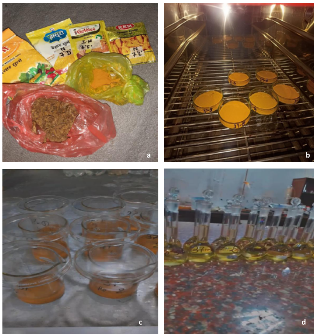
Figure 1. Different stages of sample treatment (a. Sample collected from the market, b. Drying of sample in Hot air oven, c. Acid digestion of sample, d. Sample prepared after digestion for AAS)
