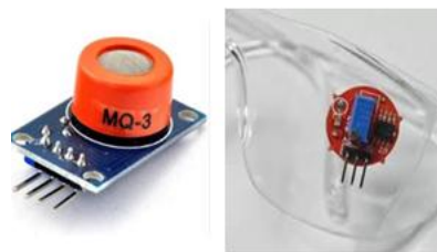
Fig. 3: MQ3 sensor for alcohol detection and Eye-blink sensor for drowsiness detection.
