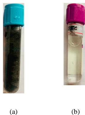
Figure 6 : Bagmati River water (a) before and (b) after treatment with BSC_1.0.
