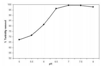
Fig. 2: Percentage turbidity removal versus the pH (at Al/Si =5, OH/Al=2.5 and PASiC dose =2.5 mg/L).
