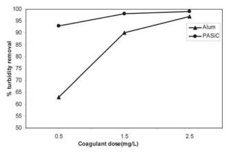
Fig. 8: Comparison of coagulation efficiency of conventional alum salt and PASiC coagulant as a function of variable coagulant dose.
