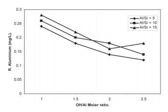
Fig. 7: Residual aluminium at different Al/Si molar ratio ( PASiC dose=2.5 mg/L).
