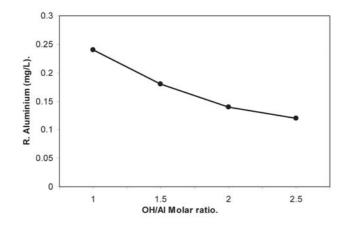
Fig. 5: Residual aluminium versus the the OH/Al molar ratio (at pH=7, Al/Si=5 and PASiC dose=2.5 mg/L).
