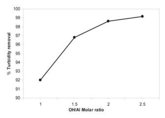
Fig. 4: Percentage Turbidity removal versus the OH/Al molar ratio (at pH=7, Al/Si=5 and PASiC dose=2.5 mg/L).
