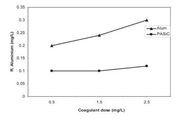
Fig. 9: Residual aluminium contents for conventional alum salt and PASiC coagulant as a function of variable coagulant dose.
