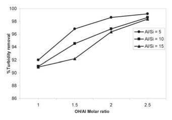
Fig. 6: Percentage turbidity removal at different Al/Si molar ratio (PASiC dose=2.5 mg/L).
