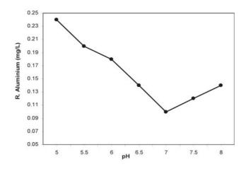
Fig. 3: Residual aluminium versus the pH (at Al/Si =5, OH/ Al=2.5 and PASiC dose=2.5 mg/L).
