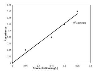
Fig.1: A plot of absorbance versus the concentration of Al in mg/L.
