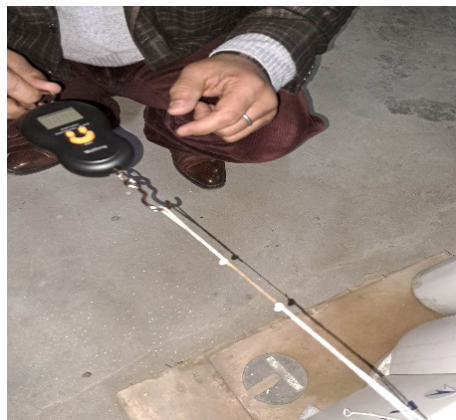
Fig. 5: Tensile strength testing of fiber
