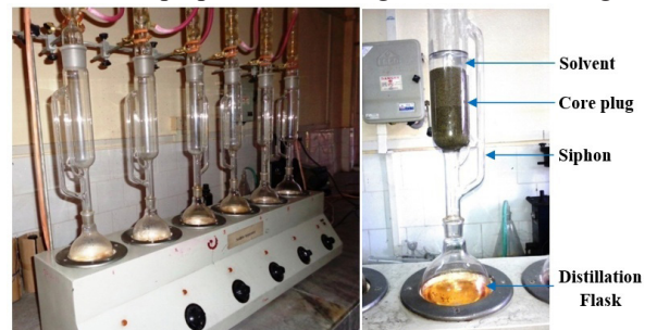
Fig. 5: Core Plugs Cleaning by Soxhlet Apparatus
