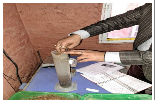
Fig. 4: Density Measurement using water replacement method
