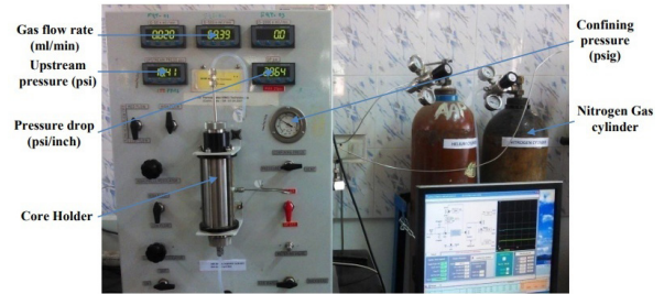
Fig. 7: Determining Air Permeability of Core Plug by NDP-605 NanoDarcy Permeameter
