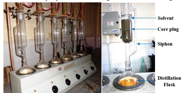
Fig. 5: Core Plugs Cleaning by Soxhlet Apparatus
