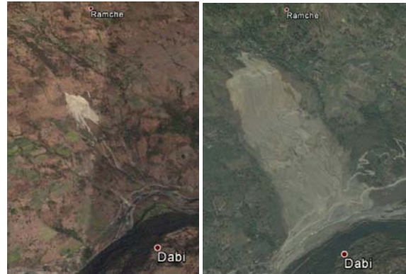
Fig. 3. Monitoring the landslide activity through satellite image (Jure landslide, Sindhupalchowk). Images of 13 Feb. 2013 (left) and 10 Aug. 2014 (right).
