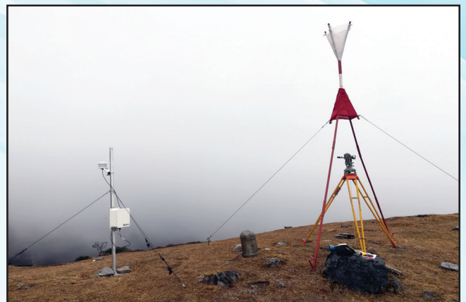
Beacon over the Wild T3 Theodolite ready for Trigonometrical leveling and triangulation and weather station during the program execution of Mt Everest Height Measurement activity.
