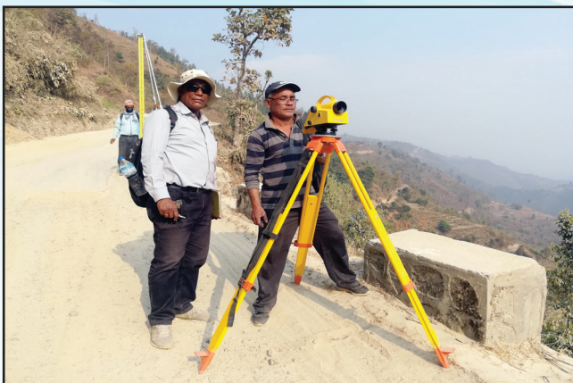
Survey Officer Mr Deepak Ratna Shakya and Mr Ram Prasad Thusa conducting Precise Leveling during the program execution of Mt Everest Height Measurement activity.
