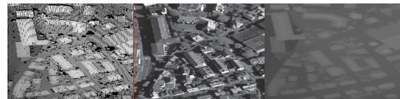
Figure: 2 Left: Laser scanner point clouds. Middle: digital aerial image. Right: Laser scanner DSM.
