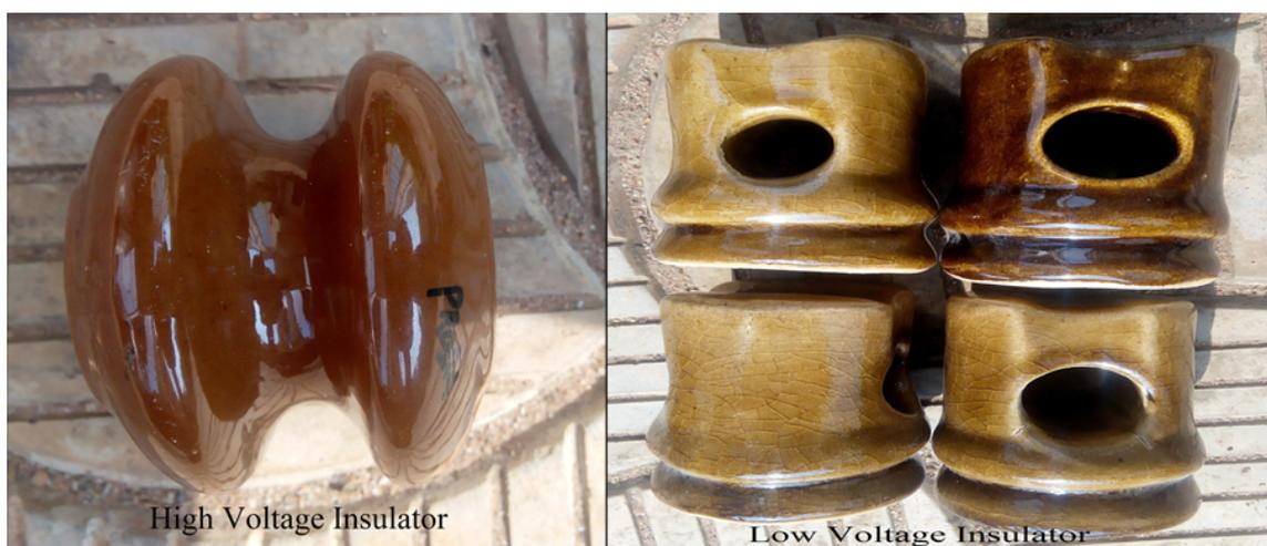
Figure 3: High and low Voltage Insulators.
