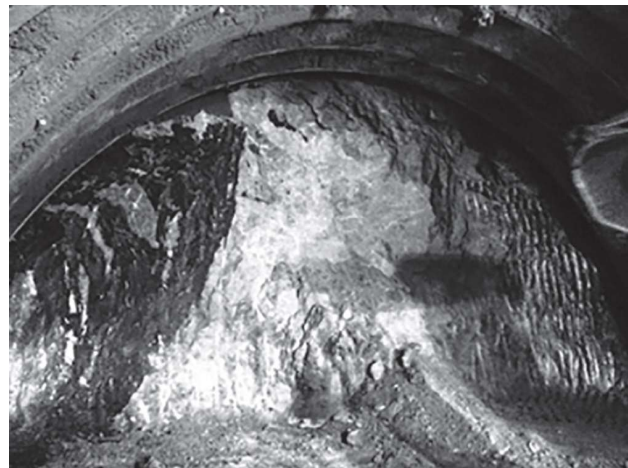
Figure 1: MT is exposed on the left in phyllite of Robang Formation at right
