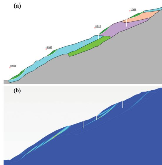
Fig. 6: Failure surfaces obtained from different methods a) LEM, b) SRM.
