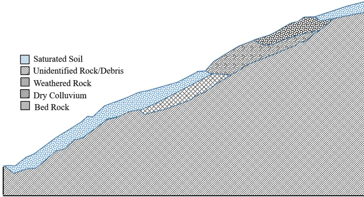
Fig. 5: Geometry and simplified subsurface layer used in analysis.
