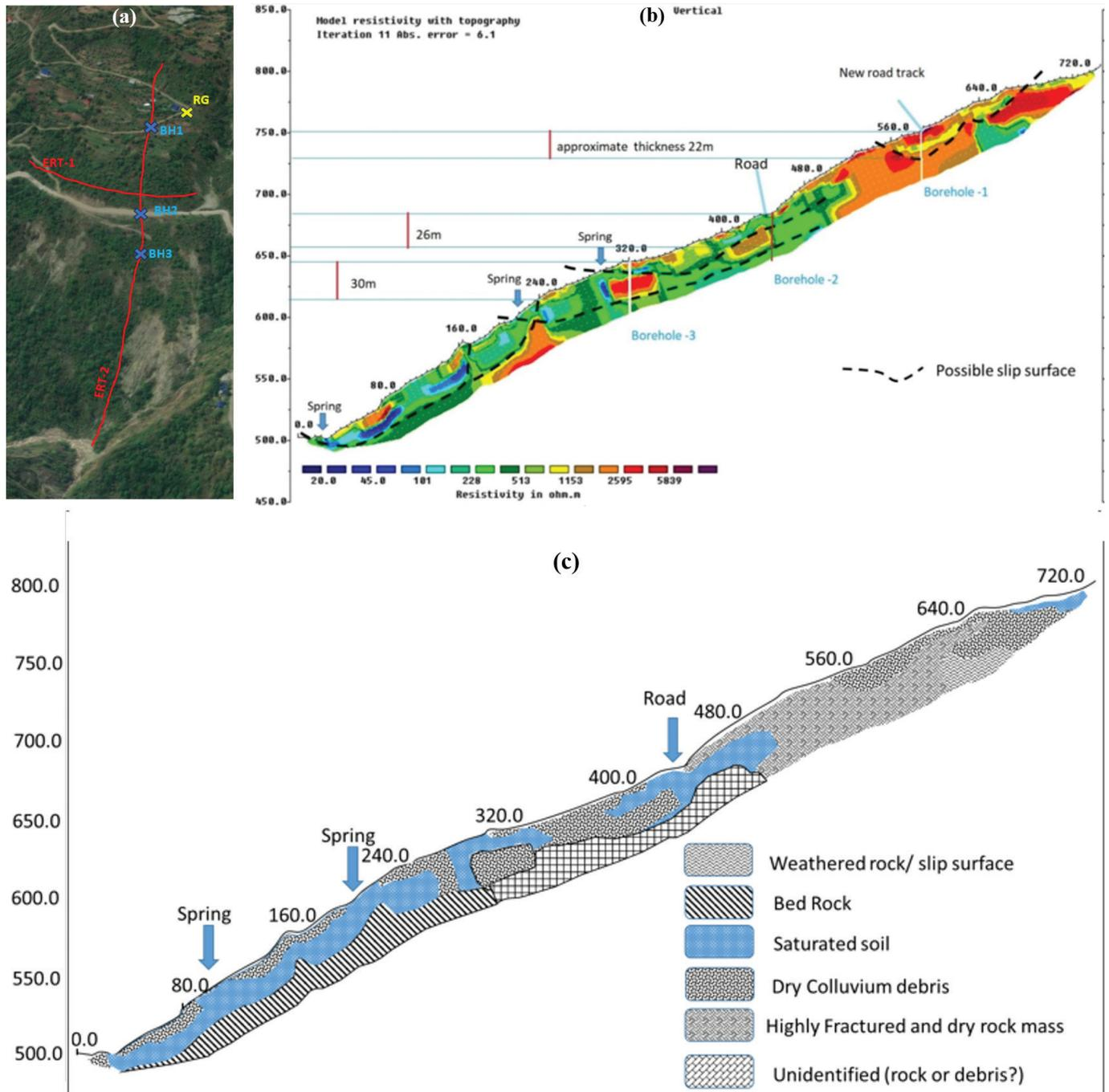
Fig. 4: Geophysical survey (a) Layout, (b) Resistivity profile, and (c) Interpreted subsurface strata.
