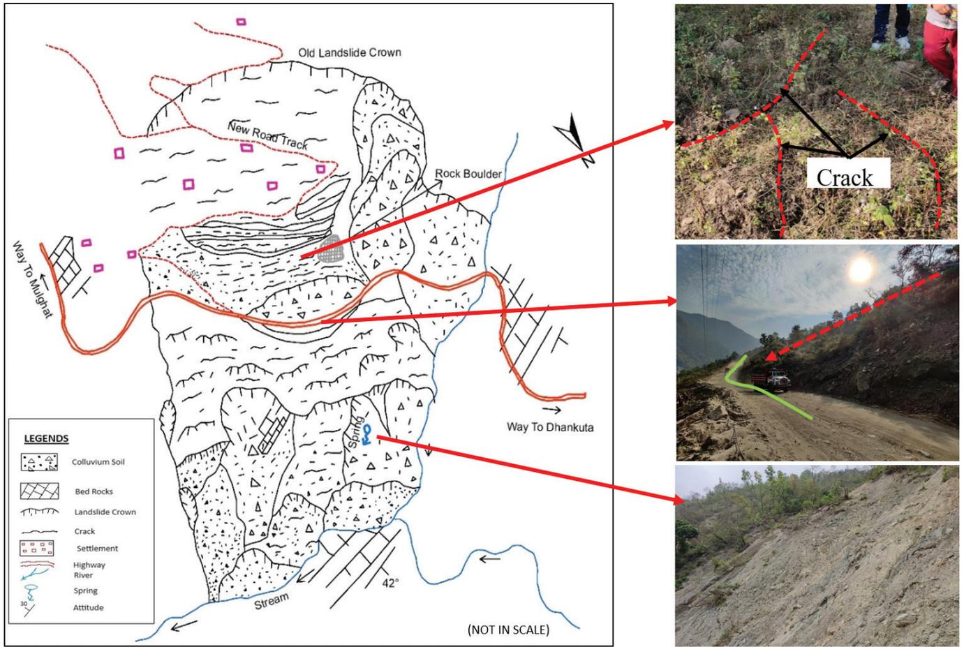
Fig. 3: A sketch showing engineering geological features of the landslide including visible slope movements.
