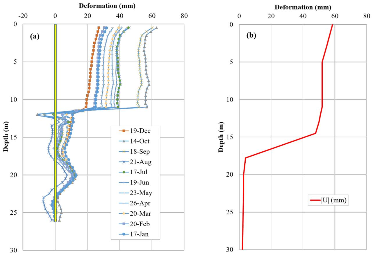
Fig. 7: Deformation pattern obtained from a) Slope monitoring, b) FEM analysis, at BH3.
