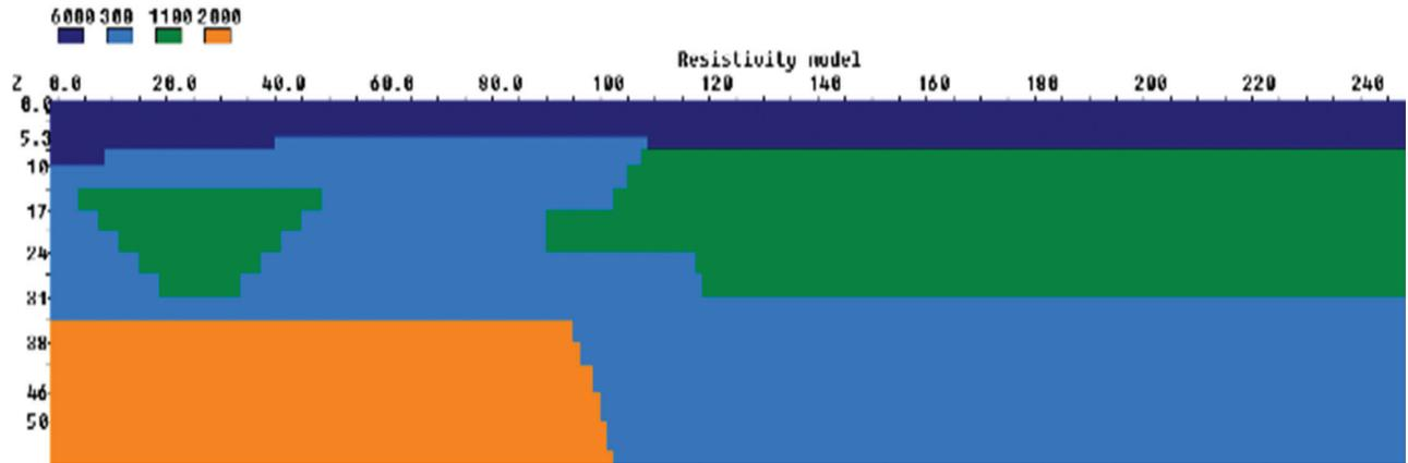
Fig. 6: Resistivity model for the collapse mass II.
