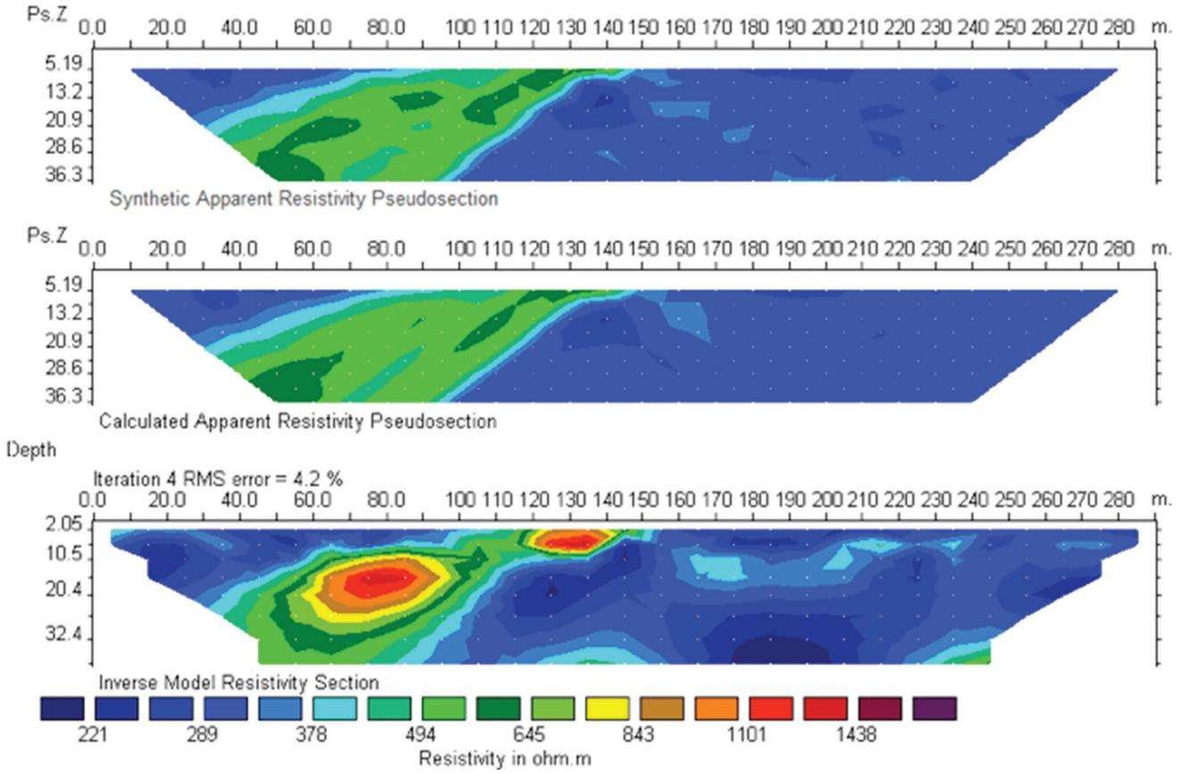
Fig. 4: Inverse resistivity sections for the collapse mass I at 5% noise level.
