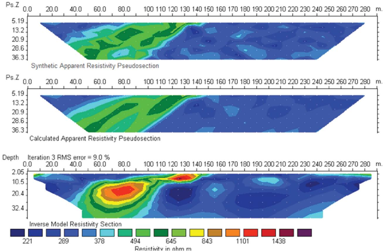
Fig. 5: Inverse resistivity sections for the collapse mass I at 10% noise level.
