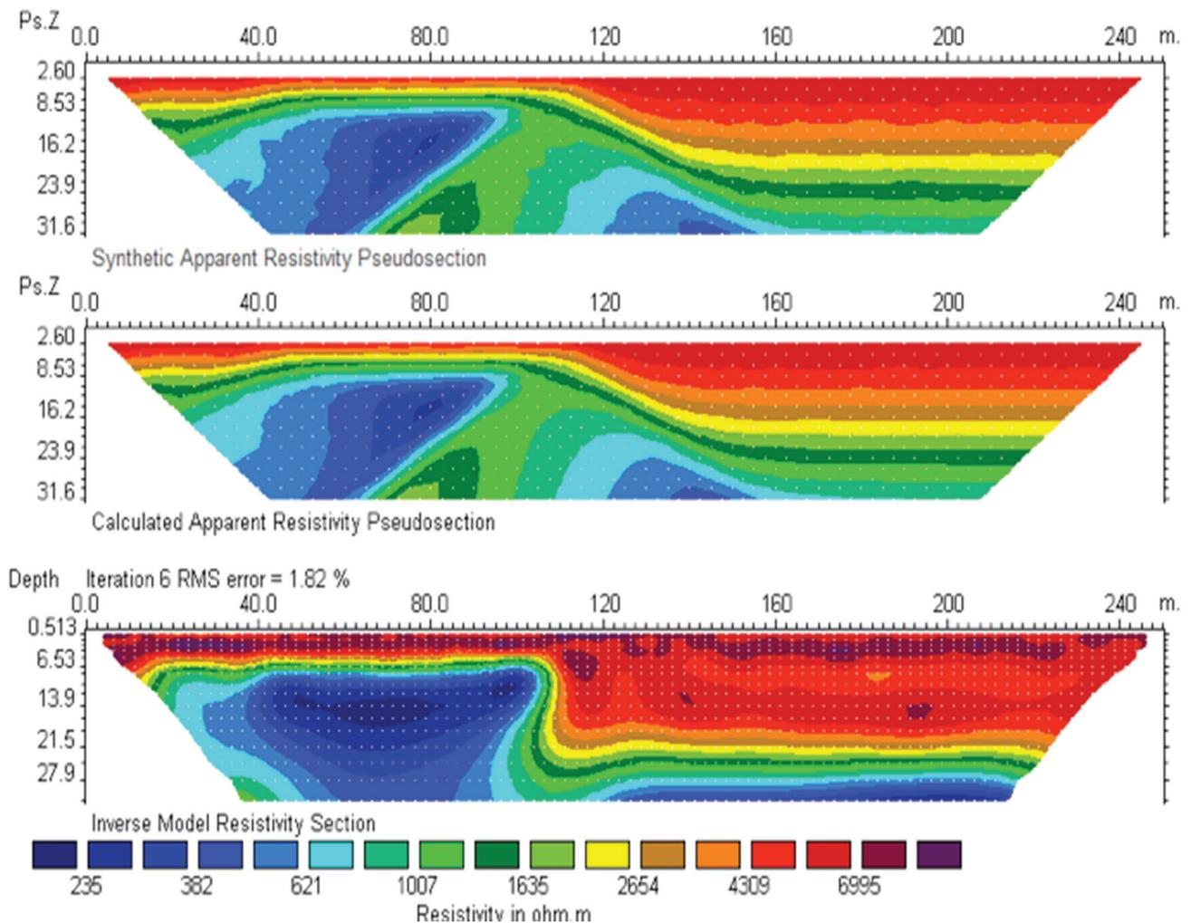
Fig. 7: Inverse resistivity sections for the collapse mass II at 2% noise level.
