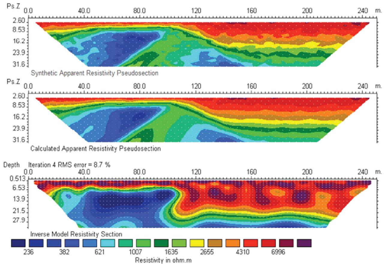
Fig. 9: Inverse resistivity sections for the collapse mass II at 10% noise level.
