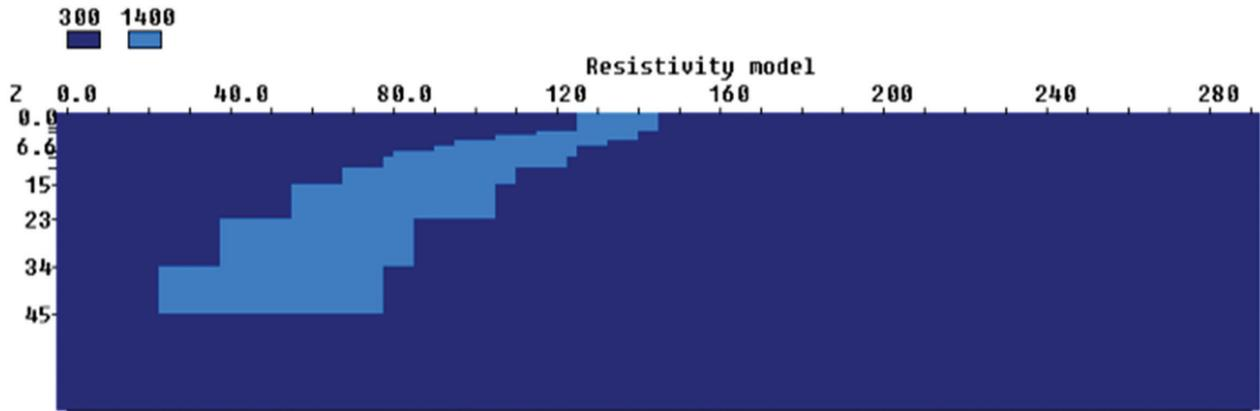
Fig. 2: Resistivity model for the collapse mass I.
