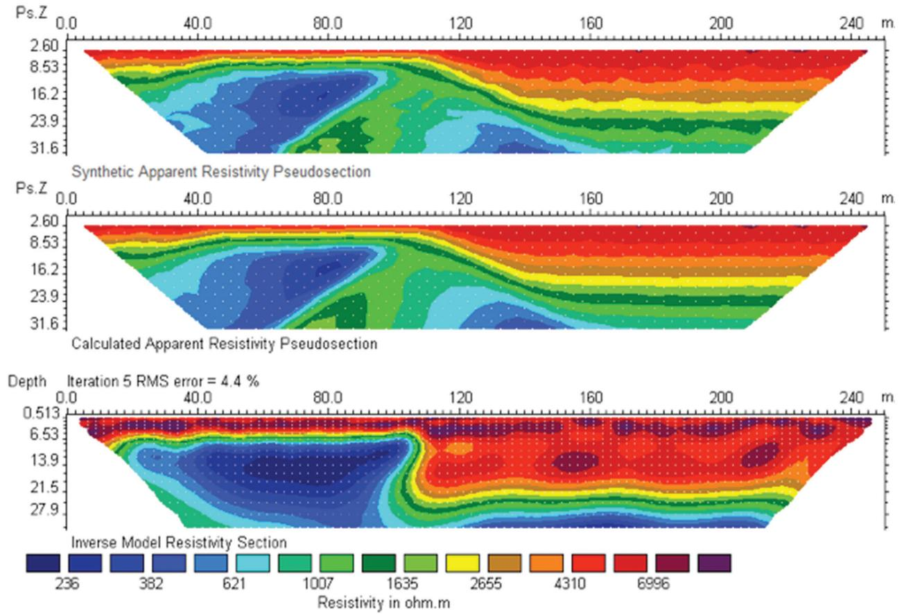
Fig. 8: Inverse resistivity sections for the collapse mass II at 5% noise level.
