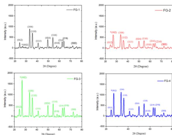
**Fig. 2:** XRD patterns of FG composites.
