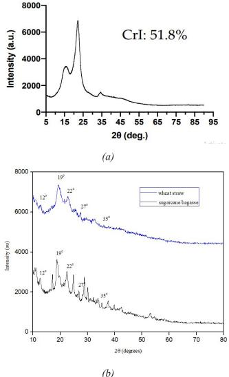
*Figure 2*: *XRD analysis of (a) commercial cellulose (b) extracted cellulose*
