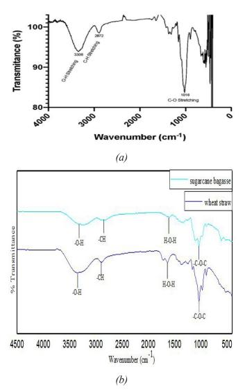
**Figure 1**: FTIR analysis of (a) commercial cellulose (b) extracted cellulose
