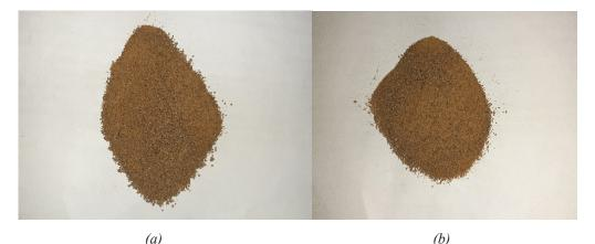
Figure 3: Extracted cellulose (a) Sugarcane bagasse (b) Wheat straw
